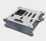
The RPCU is provided with two independent circuits (primary and secondary), based on two different (in density and reliability) FPGAs. In nominal conditions the primary circuit implements the data routing among the cameras and between the cameras and the spacecraft. The secondary circuit is based on a smaller density
